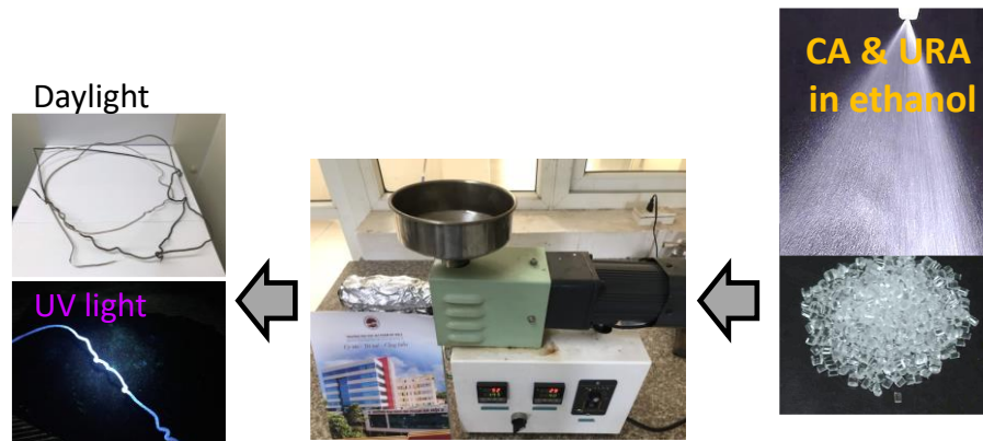
Figure 1. A thermal extrusion method to prepare photoluminescent polycarbonate composites.
