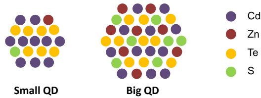
Figure 4. Quantum dot model represent the effects of size on the incorporation of Zn^{2+} and S^{2-} ions into the crystalline structure.
